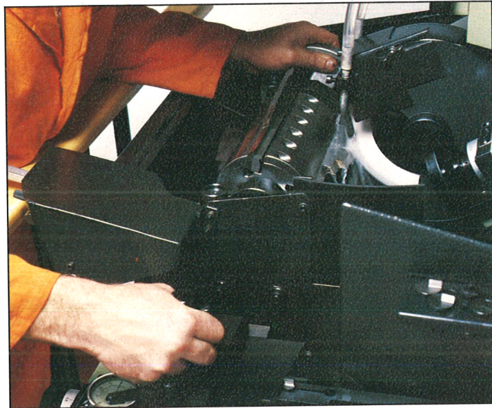
Effortless grinding and absolute accuracy are guaranteed by the floating linear table (on Model 931).
