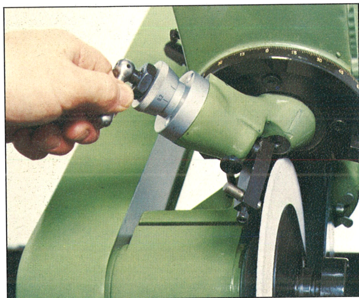
Wheel dressing is carried out in absolute safety well above grinding wheel, coolant, swarf and cutters. Angle dressing of the wheel can be achieved to within 1° accuracy.
