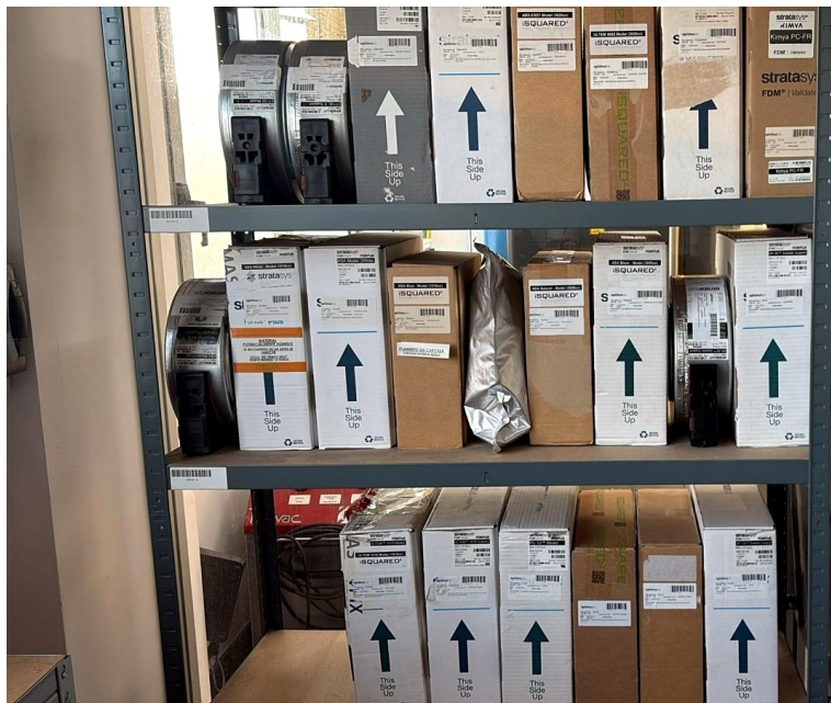
Part of the material stock — ULTEM 9085 and 1010, ABS-ESD7, PC-FR, ASA and soluble supports.
