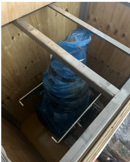
Inside crate 7/9: head sealed in HSD's blue VCI bag, bolted to the steel transport frame.
