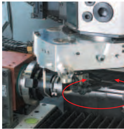
QWD 760/750 CNC-controlled E-axis
