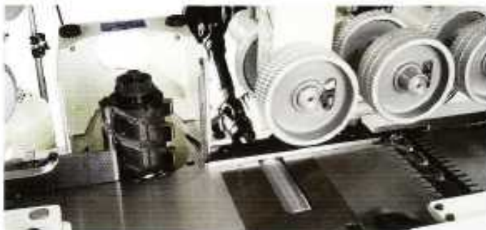
Powered feed rollers on working table to process wet timbers.
