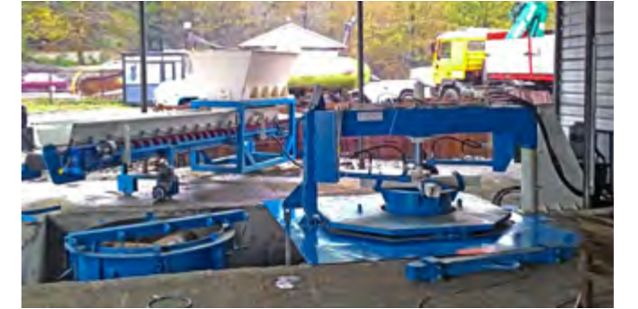
Gürcistan - ZIM B 1200 Beton Baca Üretim Tesisi Georgia - ZIM B 1200 Concrete Manhole Production Facility
