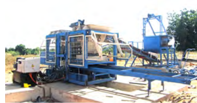
Nijer - ZIM 412 Beton Parke ve Blok Üretim Tesisi Niger - ZIM 412 Concrete Pavers and Block Production Facility
