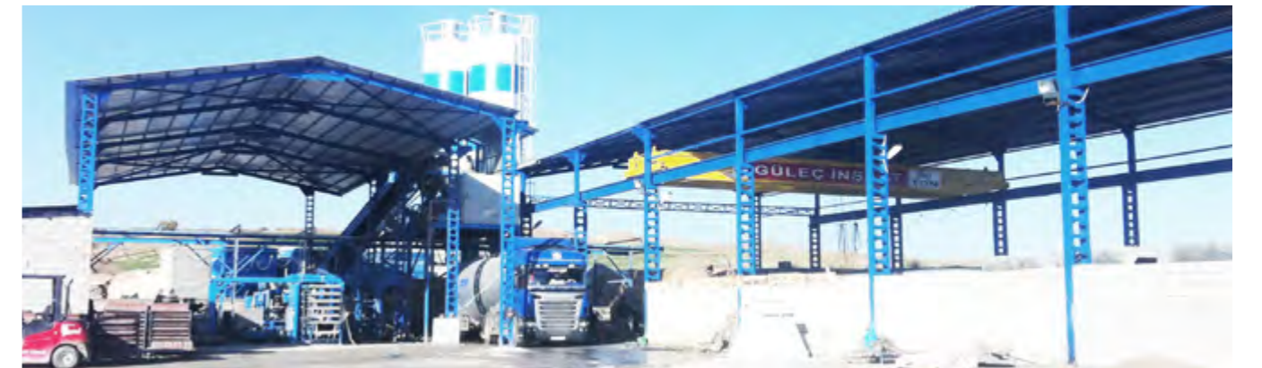
Türkiye - ZIM 1230 L Tipi Beton Parke ve Blok Üretim Tesisi + ZIM A 3000 Beton Boru Üretim Tesisi Turkey - ZIM 1230 L Type Concrete Pavers and Block Production Facility + ZIM A 3000 Concrete Pipe Production Facility
