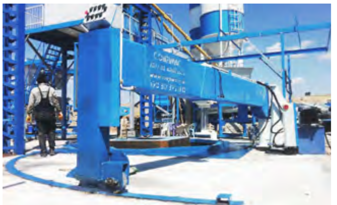
Türkiye - ZIM A 3000 Beton Boru Üretim Tesisi Turkey - ZIM A 3000 Concrete Pipe Production Facility
