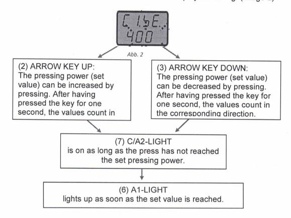
→ After 3 seconds the display returns to the initial display. (See image 1) The set pressing power is automatically saved.
