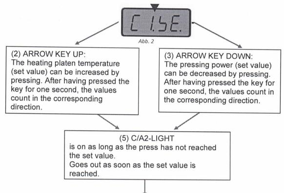
→ After 3 seconds the display returns to the initial display. (See image 1) The set heating platen temperature is automatically saved.
