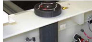
Easy access to filter The top operated developer filter housing allows the filter to be easily removed, eliminating the need for emptying the tank prior to filter removal.
