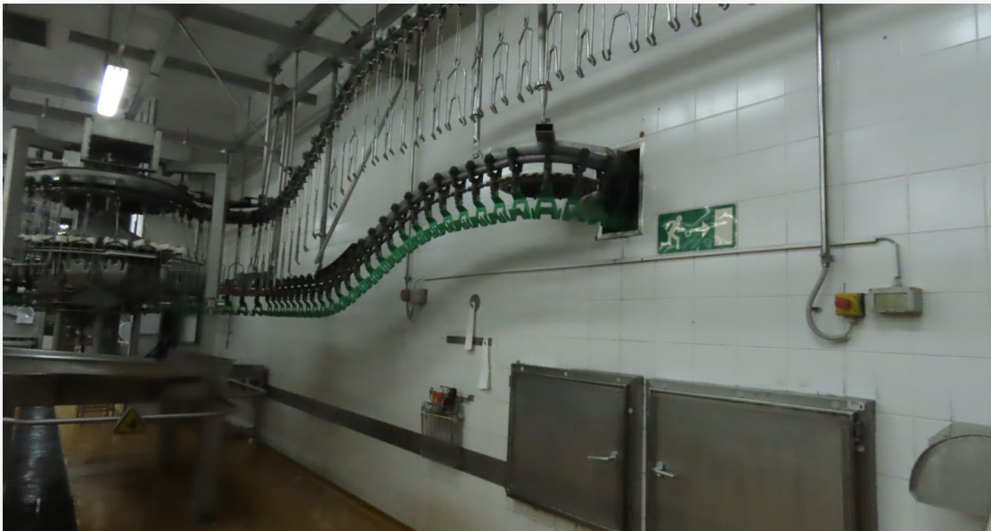
Picture 14: Return of empty OHC (from tunnel back to evisceration)
