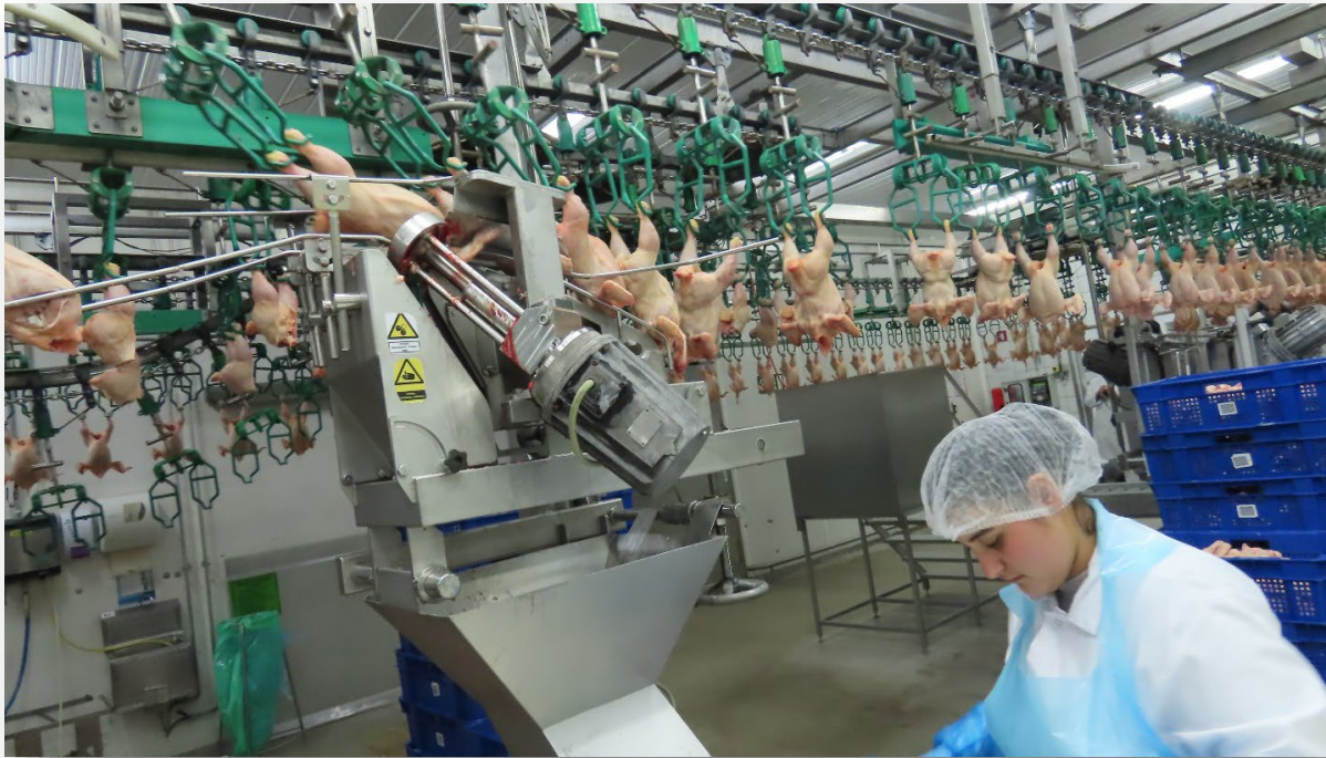
Picture 45: Chick Way module 3: the first and the second joint (third joint) of wings / complete wings
