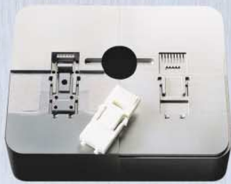
Mold for phone connector Material: Copper/Steel Surface finish: CH 22/Ra 1.26 \mu\text{m} Precision: \pm 0.0002 in Technology: Micro-machining
