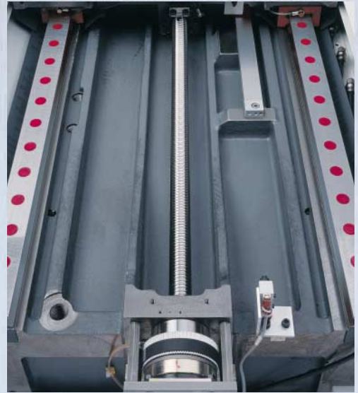
Large oversized ballscrews and linear guideways
