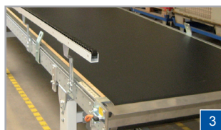
Small-roller gibs to support wide parts
