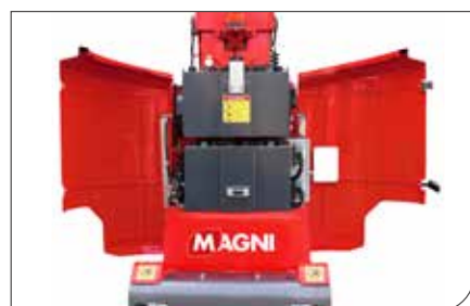
Facilitated opening for maintenance
