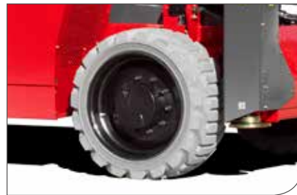
Non-marking wide solid tyres for better stability and grip
