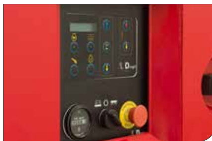
Ground control panel
