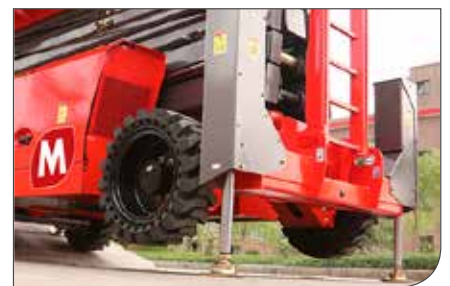
Hydraulic stabilisers with automatic levelling
