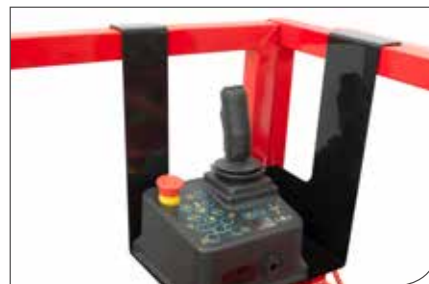
Ergonomic and removable control panel
