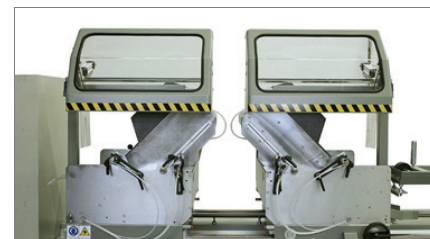
Tilting of the moving cutting heads
