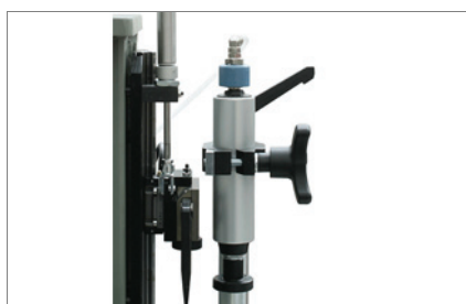
Electronic profile thickness gauge
