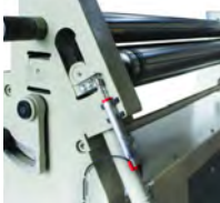
Standard Hydraulic Movement of Back Roll
