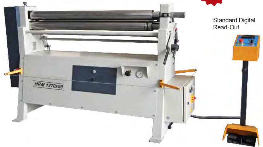
Standard Hydraulic Movement of Back Roll
