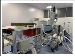
Main purpose: to insert the static electric on PP melt blown cloth
