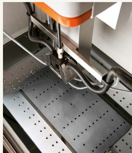
The reference holes machined under these conditions of stable temperature can achieve a positional accuracy of \pm 3 \mu\text{m} .
