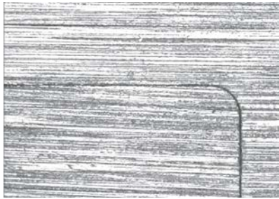
Mold insert mating face (enlarged 400 times)
