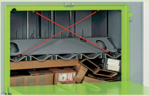
Robust: The press plunger is guided on both sides
