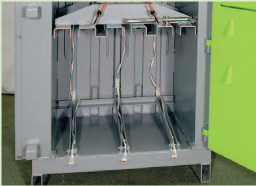
Press plunger and ejector
