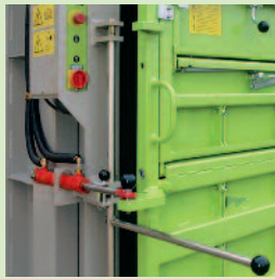
The hydraulic door opener (option)
