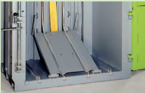
Easy to operate: The ejector
