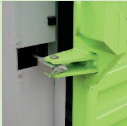
The hydraulic door opener
