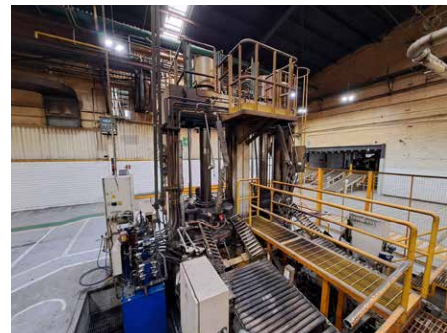
Lot. 119: GUILIN RUBBER MACHINERY FACTORY Steam-powered Hydraulic Tire Curing Press, Product No. 20061004, GUL4 Series, Year 2006
