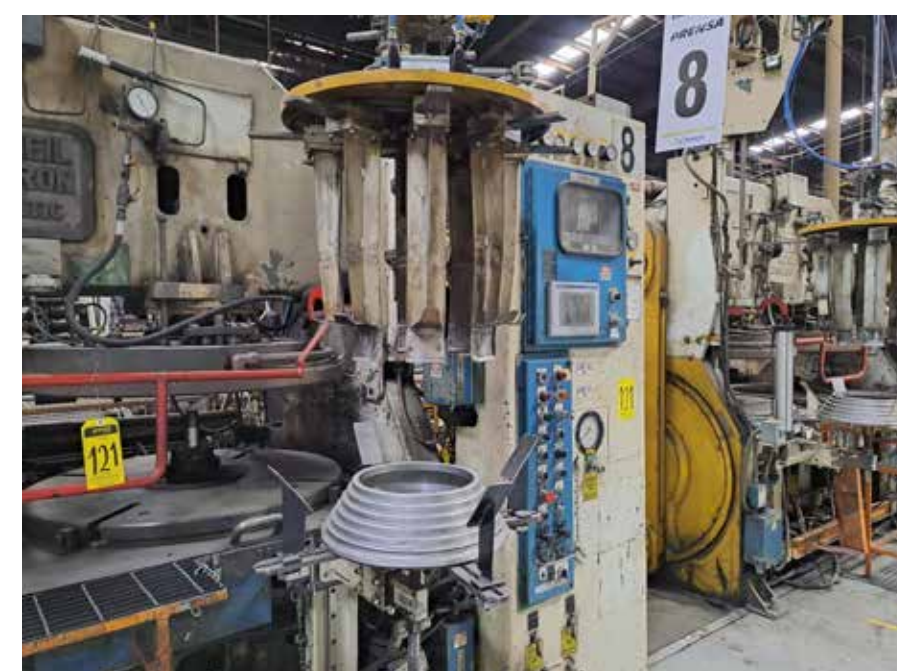
Lot. 121: MC NEIL AKRON Steam Vulcanizing Press, Model 300-4215PM-16, Serial Number BP708555277, with a maximum pressure of 300,000 lbs, mechanical clamping force: 300 metric tons, nominal platen size: 42"
