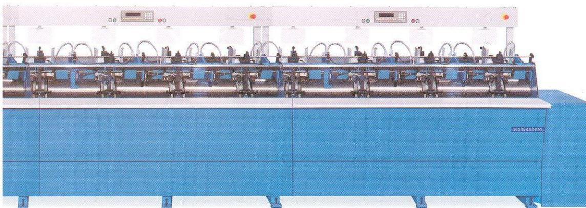
The **electronic operating element** on Sprinter 7011 consists of an LED-display with plain text information for missing and double sheets, an **Opticontrol**, ACC and a **printed mark verifier**. An on-off switch, a reset button, signal lamps, a tip-button for the setup operation and an emergency switch complement the central operating station.
