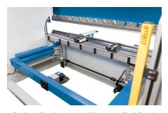
Option: Back gauge with controlled R axis
