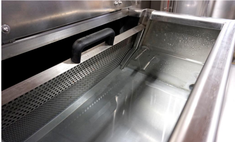
Photo: Filter sieve protect pump from mechanical debris.
