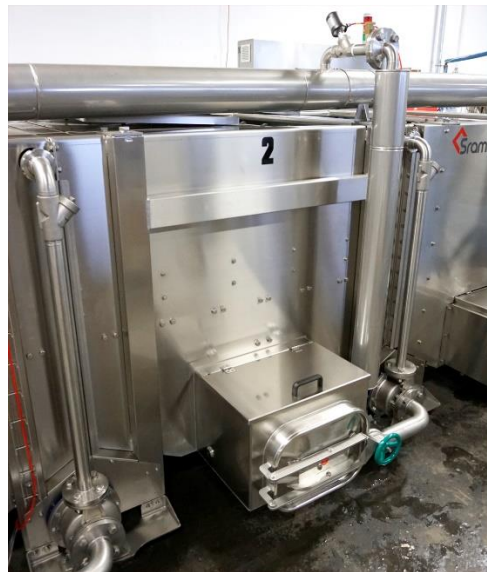
Photo: Individual modules are screwed together and they can be disassembled.
