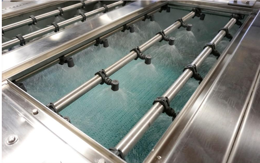
Photo: Spraying nozzles positions are precisely defined, and they are easy accessible.
