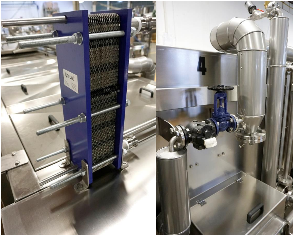
Photo: Heat exchanger and stem injection is used for process water tempering.
