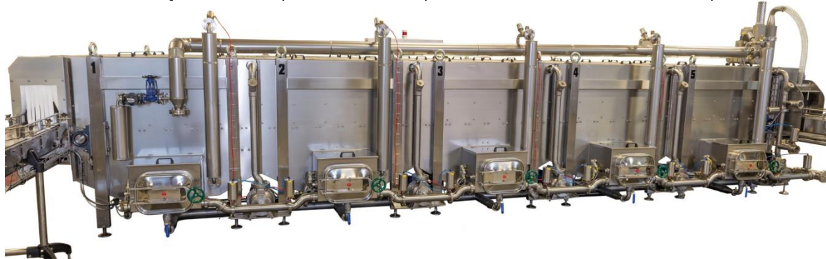
Photo: Tempering tunnel is composed more modules
