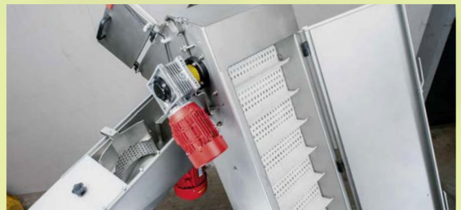
The diagram shows the SA400-RM75 with open doors and centrifugal mill removed
