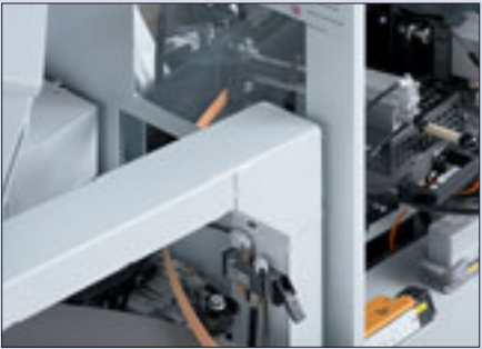
Automatic edge infeed device (optional) Automatic edge infeed device for fast change over between different coiled materials.
