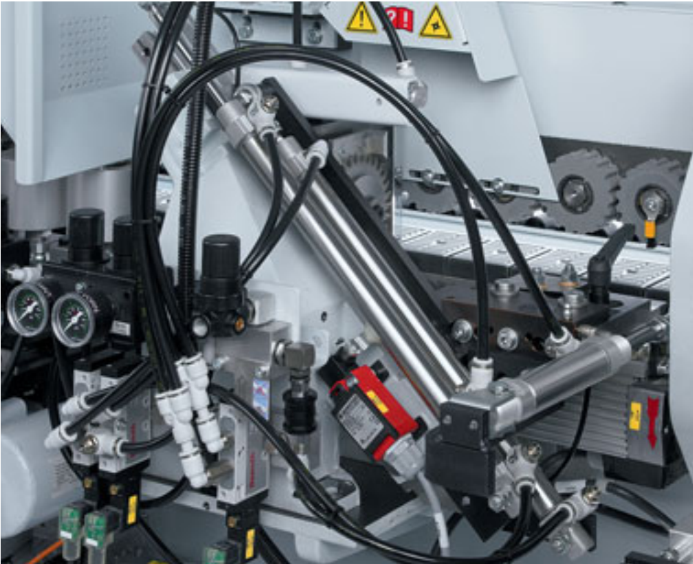
End-trimming unit Precise end-cut through a strong end-trimming unit, equipped with THK guides. Chamfer/straight adjustment by easily tilting the unit. Pneumatic adjustment.
