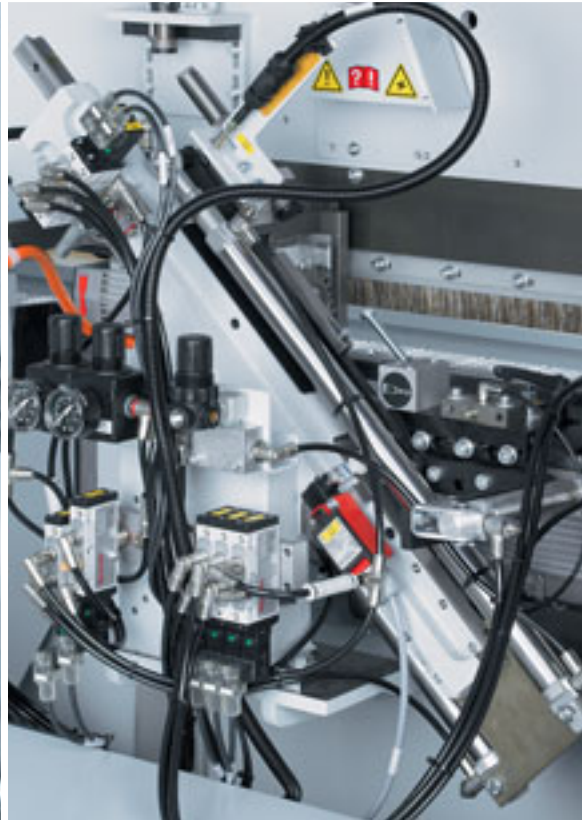
End trimming unit Perfect cutting by the end trimming unit using rigid high-precision linear guides and the workpiece gap optimization (optional) package to achieve higher output in the same processing time. Soft-touch for optimal end trimming results even at high speeds.
