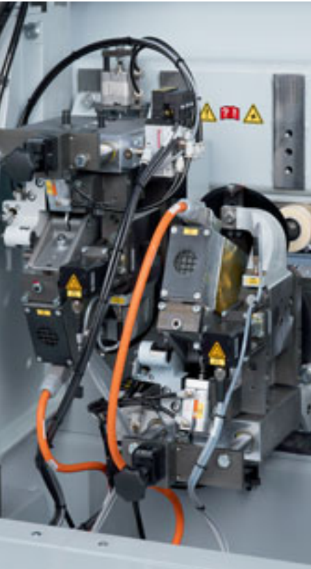
Multistage trimming unit MS 40/45 (optional) Fully automatic adjustment between 3 different profiles by means of servo motors.
