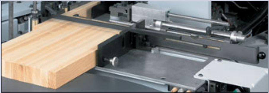
Extra wide magazine (optional) Extra wide magazine with high capacity for fixed length strips and optimum access to reload.
