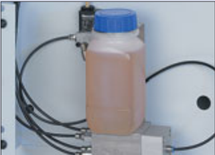
Central lubrication unit To lubricate the feed track guidance system to guarantee precision and a long life of the conveyor chain.
