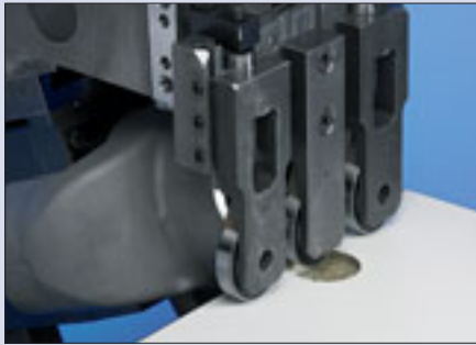
Nesting package (optional) Includes a multi-roller tracing device for the trimming and scraping units to compensate for hinge holes.
