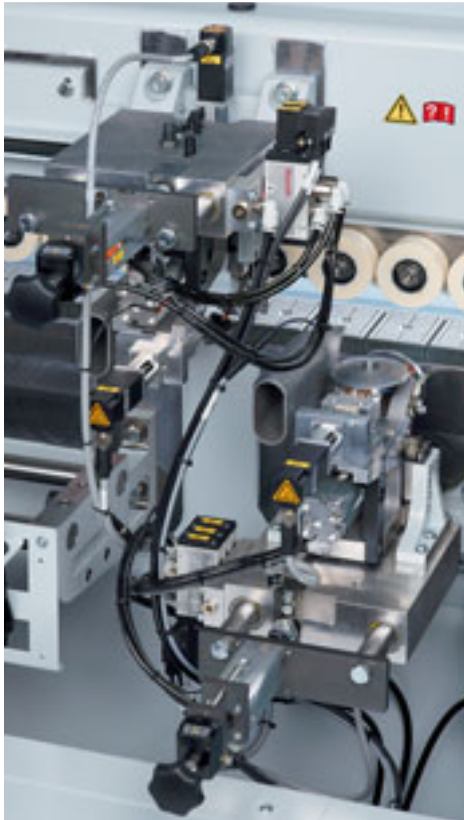
Multistage scraping unit MZ 40 (optional) Fully automatic adjustment between 2 different profiles by means of servo motors.
