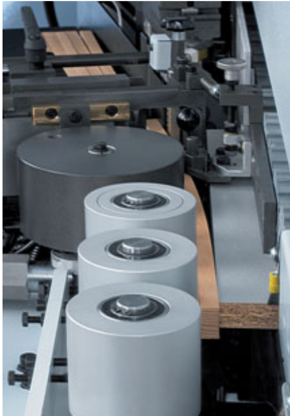
Pressure zone Heavy pressure zone (up to 15 mm) to ensure an optimum glue joint quality.
