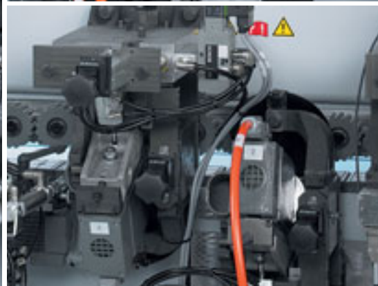
Trimming unit Trimming unit with DFC (Dust Flow Control) tooling technology for optimal extraction. Optional pneumatic or servo axis adjustment available. Multistage trimming unit MS 40/45 (optional) Fully automatic adjustment between 3 different profiles by means of servo motors.
