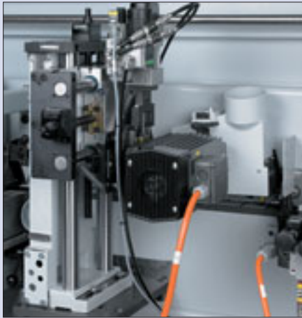
Universal trimming unit Universal unit with high capacity for grooving and profiling work. Flexible by unlimited setting options.
