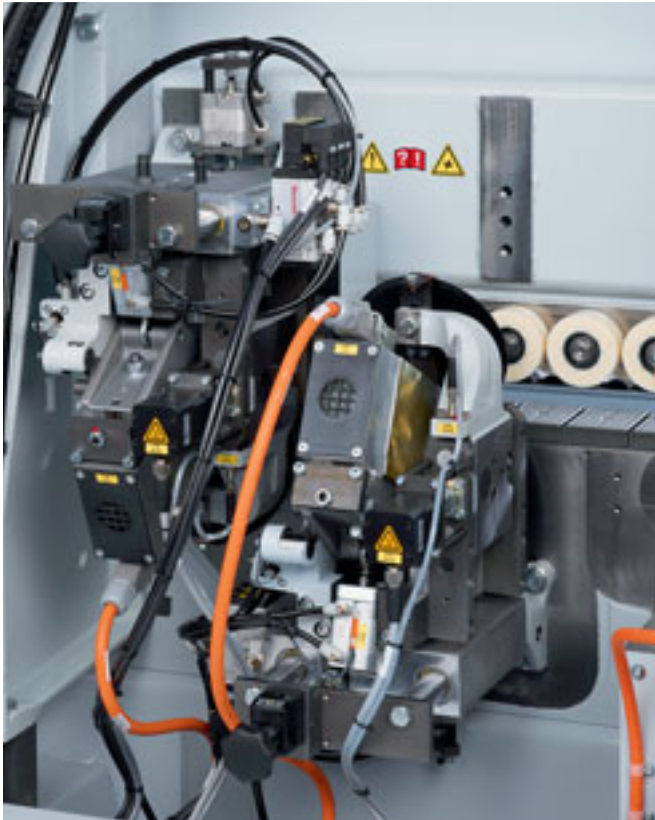
Multistage trimming unit MS 40/45 (optional) Fully automatic adjustment between 3 different profiles by means of servo motors.
