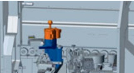
QA 45 – Manual • The application unit is filled by hand either with granulated glue, or with glue slugs • Flexible application of different hot melt adhesives, like EVA, PU or Polyolefine based glue or different glue colours
