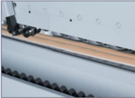
V-belt top pressure (optional) Top pressure V-belt system optionally available instead of the standard top pressure roller system.
