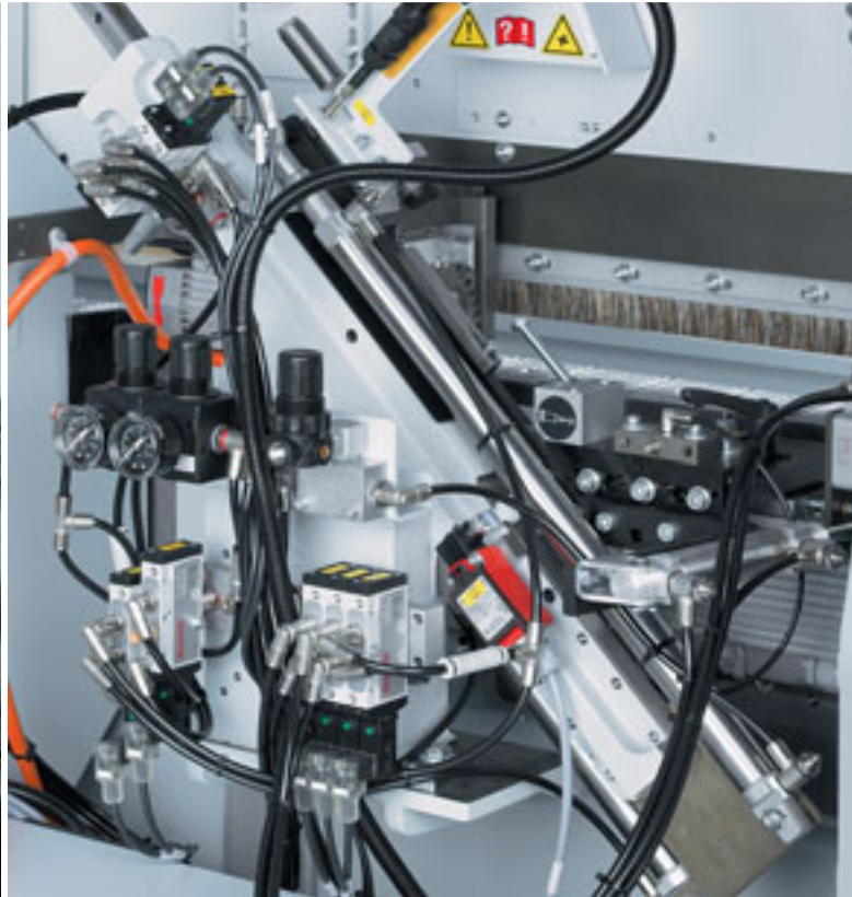
End trimming unit Perfect cutting by the end trimming unit using rigid high-precision linear guides and the workpiece gap optimization package to achieve higher output in the same processing time. Soft-touch for optimal end trimming results even at high speeds.
