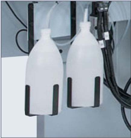
Spraying unit Separation and detergent agents for a perfect finish when processing PU-glue.
