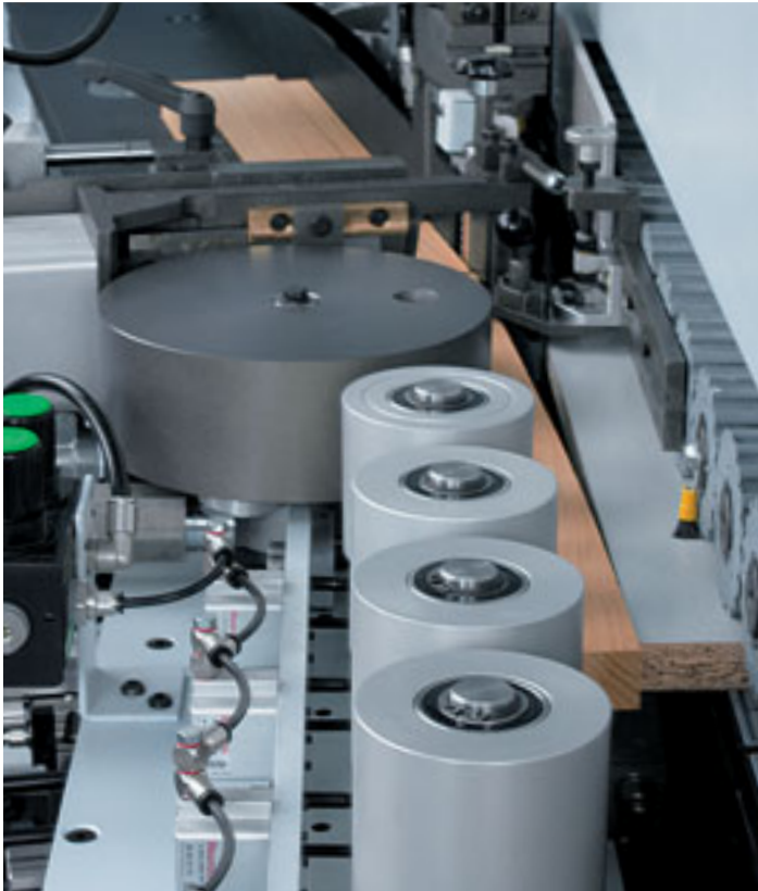
Pressure zone Heavy pressure zone (up to 20 mm) to ensure an optimum glue joint quality.
