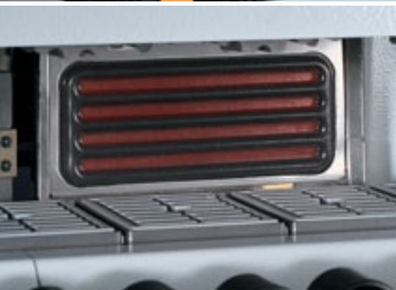
Radiant heater Strong adhesion through optimal pre heating of the workpiece.
