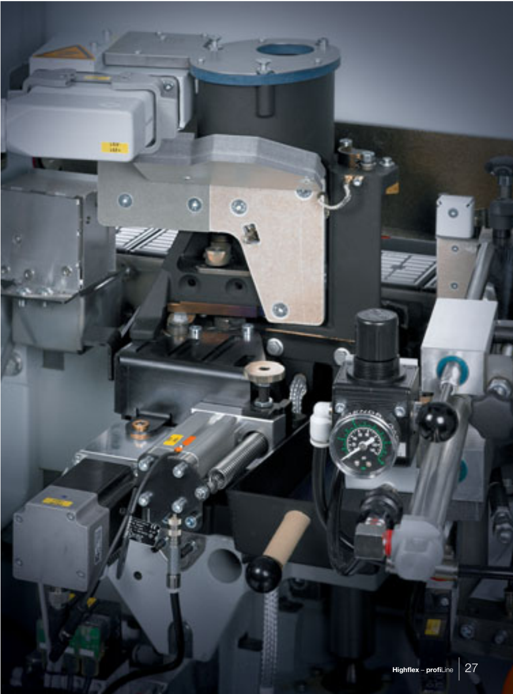
QA 45 – EVA • EVA pre-melting unit for hot melt glues • Filling capacity approx. 4 ltrs. granulated hot melt glue
