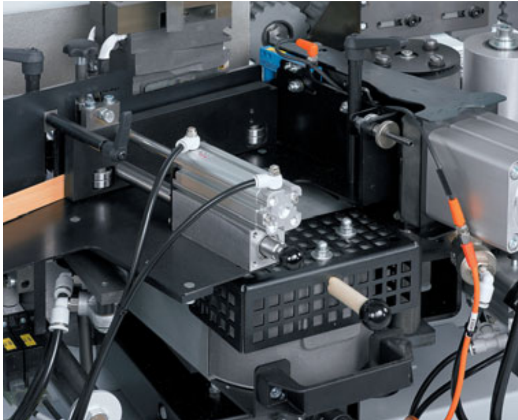
Gluing unit and magazine Coil and automatic strip magazine for a reliable edge material supply. Optimal glue joints, by controlling the exact amount of glue.
