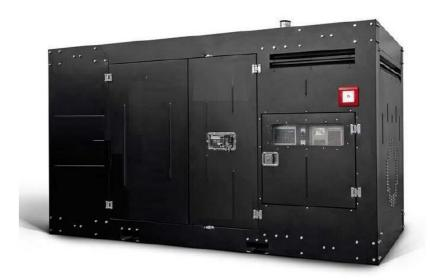
The enclosure is designed to guarantee 55db(A) at 7 meters in a free field, and optimum performance in all conditions. Fully designed on modular principles, the enclosure permits an easy on-site repair, thanks to the easy interchangeable panels.
