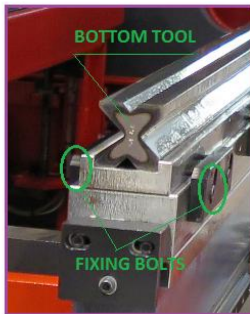
Figure-34: Changing the bottom tool 1.2.b. fixing bolts on the bed.
