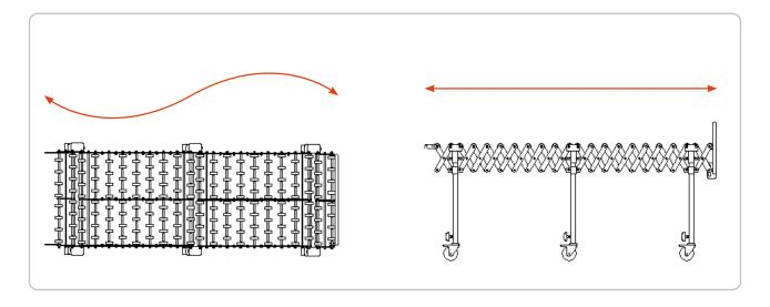
1. The height of the roller conveyor can be adjusted, and when transporting goods, it is possible to have an inclined position. You can adjust the height of the feet individually by adjusting the leg handle.
