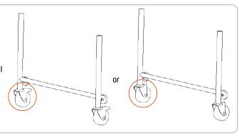
3. Take the roller track out of the box and attach the feet.
