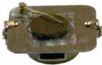
Fig. 6-4. Sample fixed on a substrate with a spring contact with a double-sided adhesive tape, substrate placed on a non-magnetic holder
