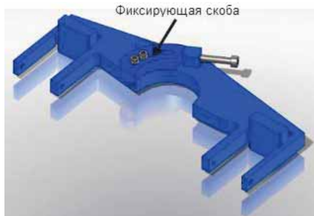
Fig. 2-14. Bracket of videomicroscope. The fixing bracket is unlocked
