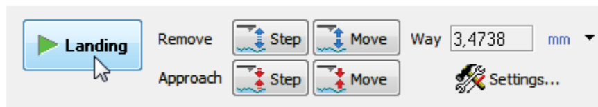
Fig. 8-9. Control panel of the Approach window
