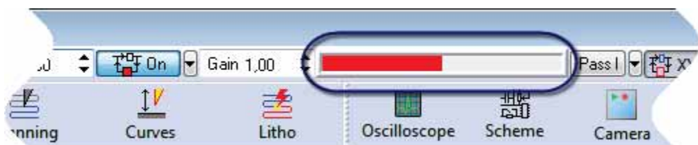
Fig. 8-11. Scanner extension indicator after approaching
