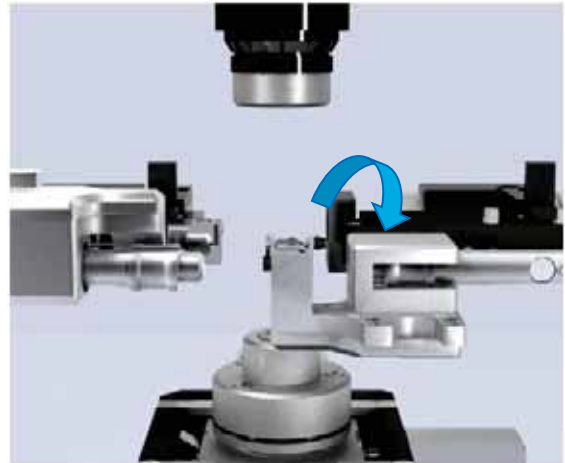
Fig. 1-7. AFM head in position for exchanging the probe
