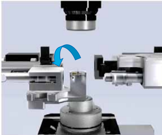
Fig. 1-6. STM head in position for exchanging the probe
