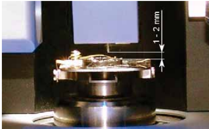
Fig. 6-31. The distance between the probe tip and the sample surface is 1–2 mm
