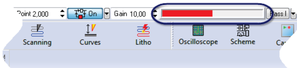
Fig. 7-6. Scanner extension indicator after approaching
