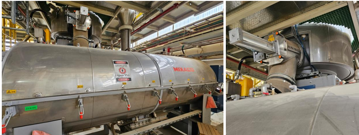
Left: Cooling Mixer – special discharge valve from hot mixer, right side the aspiration. Right: special discharge valve
