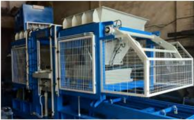
Umman - ZIM 1230 Beton Parke ve Blok Üretim Tesisi Oman - ZIM 1230 Concrete Pavers and Block Production Facility
