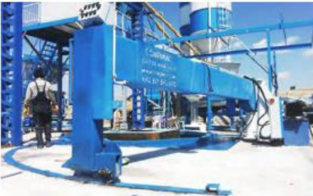
Türkiye - ZIM A 3000 Beton Boru Üretim Tesisi Turkey - ZIM A 3000 Concrete Pipe Production Facility
