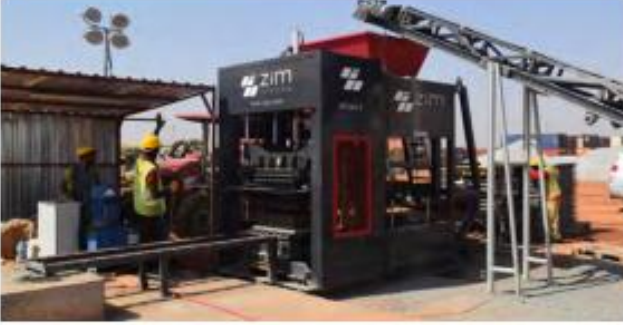
Nijer - ZIM 8 Beton Blok Üretim Tesisi Niger - ZIM 8 Concrete Block Production Facility
