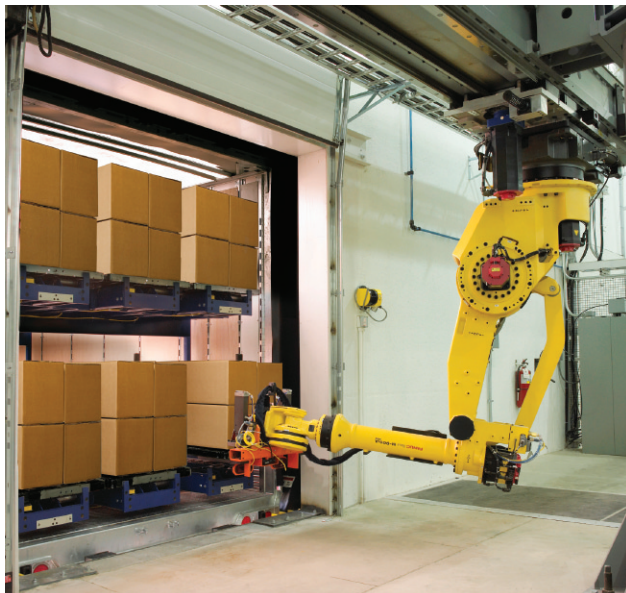
Ceiling mounted M-900 i A/350 unloading trucks.
