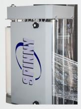
The motorized pre-stretch system, allows an efficiency of film **up** to 300%
