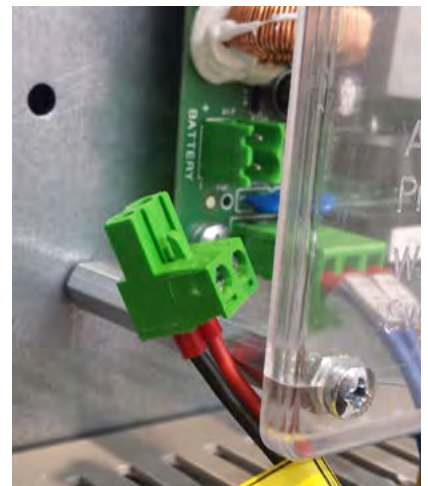
AT FIRST START-UP CONNECT CABLE 21-7 AND 21-8 FROM BATTERY -2 1G2 TO PIN X17 OF ELECTRONIC BOARD OB1 (-21K2)
