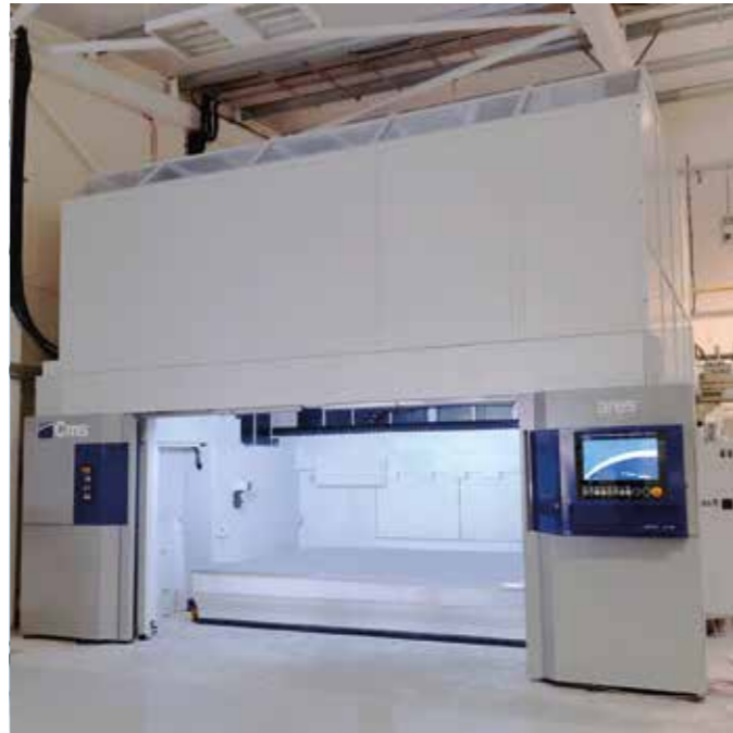
Soundproof full enclosure for dust control and for machine's lighting
