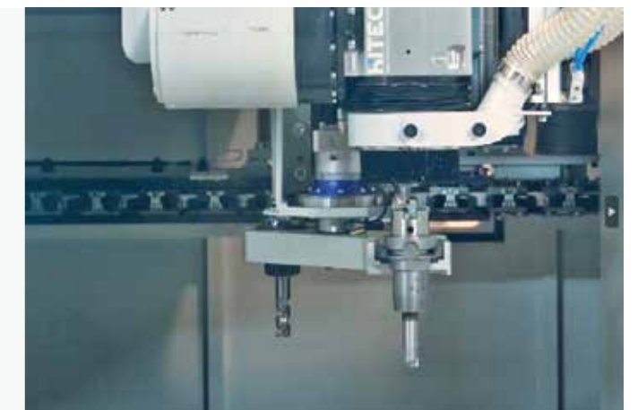
Tool-chain magazine with exchange handgrip
