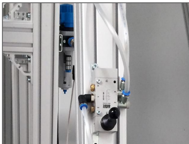
Figure 16: Manual valve for actuating fixing clamp
