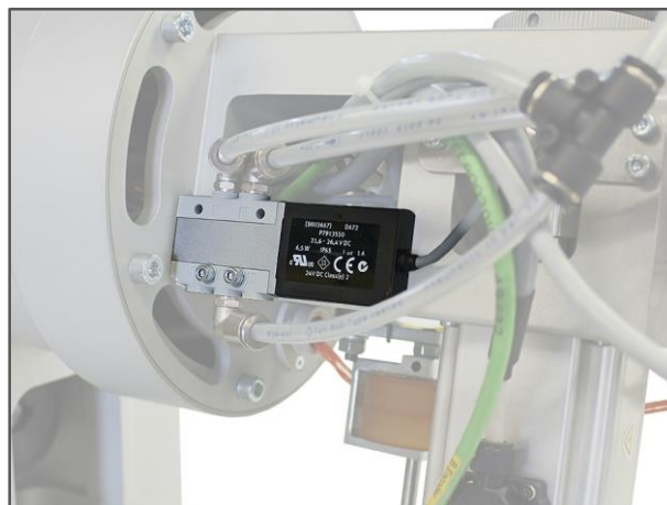
Figure 37: Cut/Loop pneumatic valve
