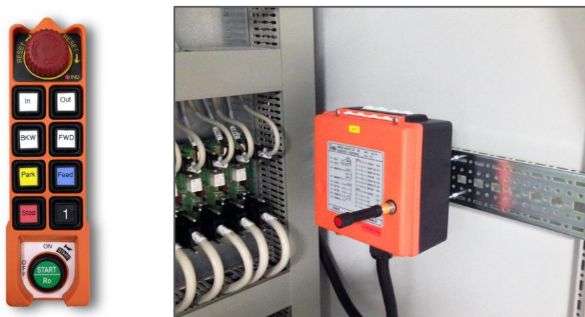
Figure 22: Left) Remote Control Commander; Right) Remote Control Receiver
