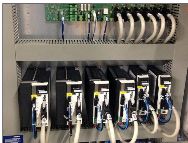
Figure 28: Servo drives, from left to right: X, Y, Z, C, B and A axes
