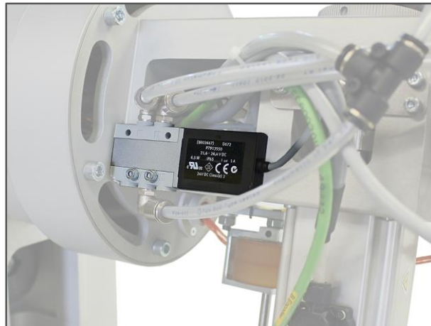
Figure 20: Cut/Loop pneumatic valve
