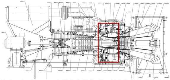
The damaged gas hoses were repaired. During final testing of the unit in September a small gas leakage was found at the #11 burner (connection of the main gas hose to the gas manifold. This could not be corrected by tightening, hence a gas hose from the replacement unit was installed.
