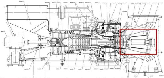
The power turbine blade 3 and honey comb segments were originally replaced by new. After the hot section damage the blades were damaged and replaced on-site by used serviceable blades from the replacement unit together with the honey combs 3 (complete guide vane 3 assembly form the replacement unit was used.
