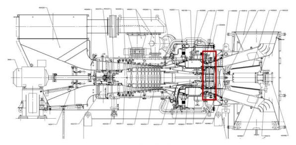
All bypass sleeves were changed to new beer jug type. Additionally the bypass sleeve blocks were modified with cups and springs from the replacement unit. The locking pin was replaced and modification with T3910 locking plate was implemented, which should stop the hot air leakages.
