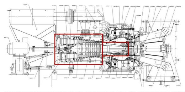
All compressor blades have been replaced with new blades which have a 5380 DP aluminum oxide anti fouling coating. After installation of the blades the rotor assembly was high speed balanced at VDL including a 3 minute overspeed run at 10% overspeed. The blade tip clearances were checked during installation.
