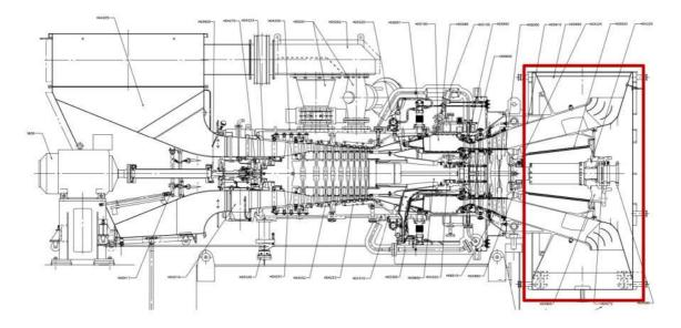
Cracks in the corners and flanges of the exhaust were repaired by the client. Additionally the insulation and the horizontal compensator were replaced by the client.
