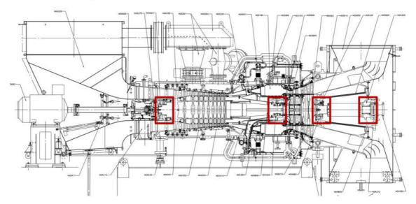
All bearing housings were cleaned from oil coking. Oil analysis revealed that although the oil has a dark color it is still in suitable condition.
