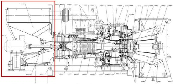
No work has been performed in the starter or flex coupling.
