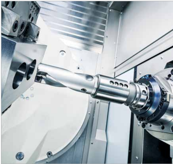
Motorized spindle 12,000 rpm (83 Nm | 61 ft-lbs)/HSK-A63 Machining on a G350
