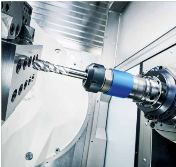
Motorized spindle 16,000 rpm (206 Nm | 152 ft-lbs)/HSK-A63 Machining on a G350
