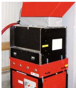
Filling with bale conditioning system (stationary use)
