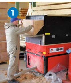
Filling with insulation sacks (mobile use)
