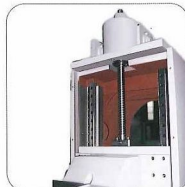
Vertical ballscrew and servo motor.
