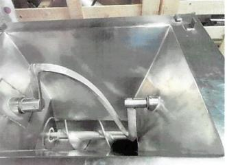
By way of mincing once and then loading into tote bins additional ingredients can go into the tote bins. The mobile tote bin loader can tip the product back into the Kilia 130 Mixer Grinder, then mix and mince out
