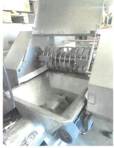
Flaked product can be fed directly into the Kilia Mixer Grinder by the Scansteel Giraffe Feeder Or if the flaked meat is in tote bins the mobile hoist can tip the tote bins into the Kilia Mixer Grinder
