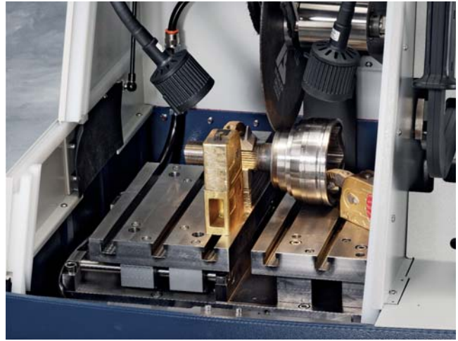
Speed vises and riser blocks provide vertical clamping forces for large and irregularly shaped samples.
