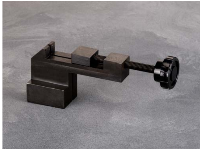
Fastener vise for longitudinal sectioning of small parts.
