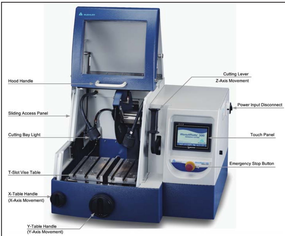
Determine cutting length by measuring the distance where (1) the abrasive wheel meets the vise table when first making contact with the sample plus the (2) length of the sample.
