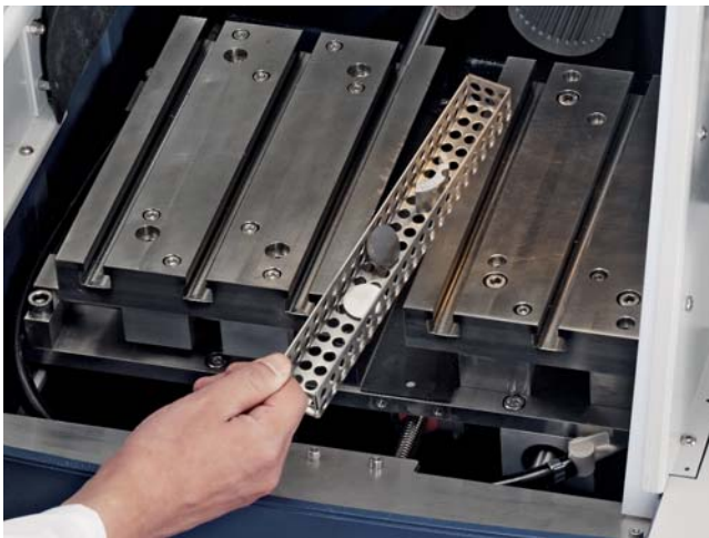
Parts tray catches small samples for easy retrieval.
