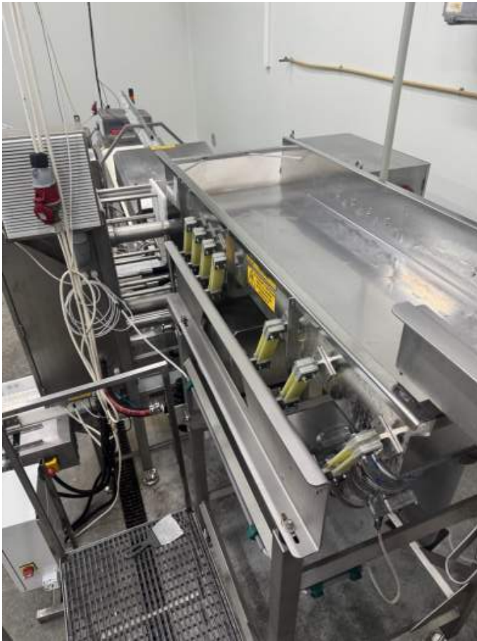
10. Vibration table for spreading berries – Best/Tomra
