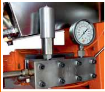
Stainless steel pump-head. Integrated cooling for plunger-seals.
