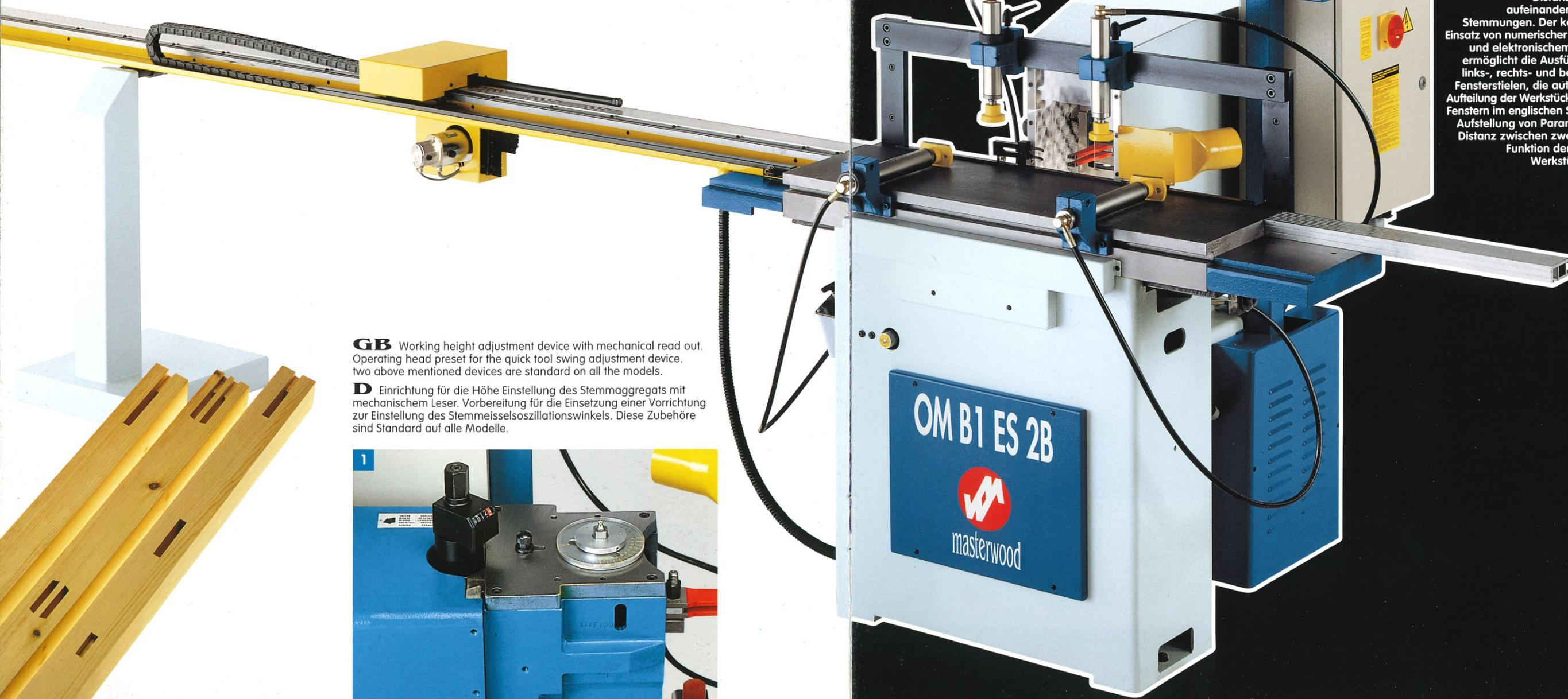
**GB** Working height adjustment device with mechanical read out. Operating head preset for the quick tool swing adjustment device. two above mentioned devices are standard on all the models.
