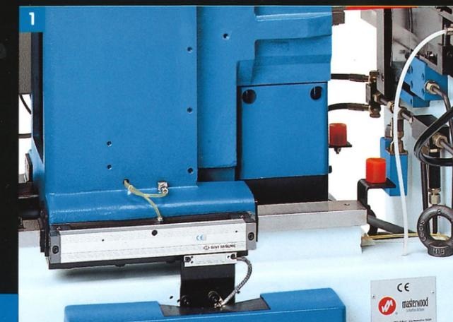
**GB** Operating head displacement and working depth handled by the control by means of an opto-electronic linear trasducer (only on OM B1 ES 2 and OM B1 ES 2B).
