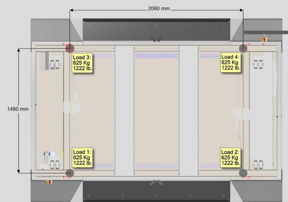
Figure 6: Leveling and Supporting Pads - Specifications
